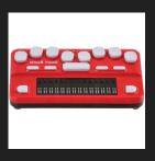
Refreshable Braille Display & Keyboard Provides users the ability to utilize eBraille as both input and output.
