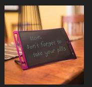
Boogie Board Jot is an LCD eWriter that allows non-verbal or speech-impaired communication.
