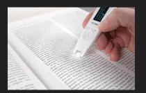
C-Pen Reader Pen Scanner reads printed text out loud; helps with dyslexia.
